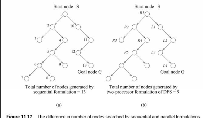
**Figure 11.17** The difference in number of nodes searched by sequential and parallel formulations of DFS. For this example, parallel DFS reaches a goal node after searching fewer nodes than sequential DFS.
