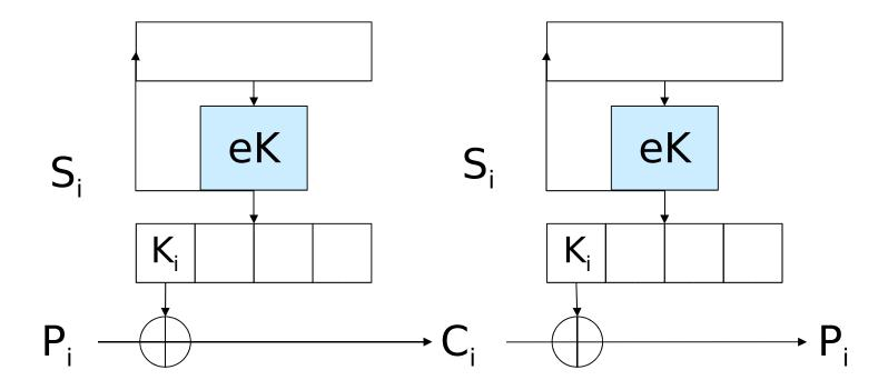
A bit error in the ciphertext affects exactly the same bit in the plaintext.
