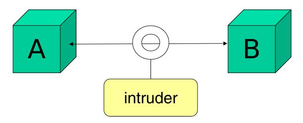
A and B communicate over an insecure channel.
