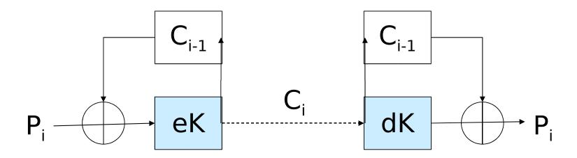
A corrupted ciphertext block  $C_i$  affects only the two plaintext blocks  $P_i$ ,  $P_{i+1}$ .
