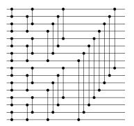
Figure 2: A Green filter on 16 channels.
