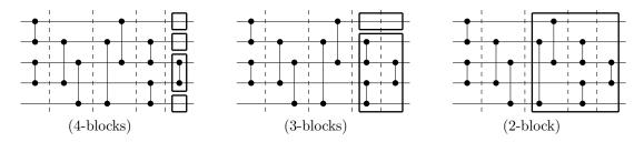
Figure 4: The 4-, 3- and 2-blocks of the sorting network  $\{(1,2), (3,4)\}, \{(2,4), (3,5)\}, \{(1,3), (2,5)\}, \{(2,3), (4,5)\}, \{(3,4)\}$ .
