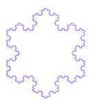
For example, to generate a Koch curve, we start with the initial (depth 0) state F signifying a forward move, i.e., a straight line. The rule for expanding to the next depth is given as a replacement rule.
