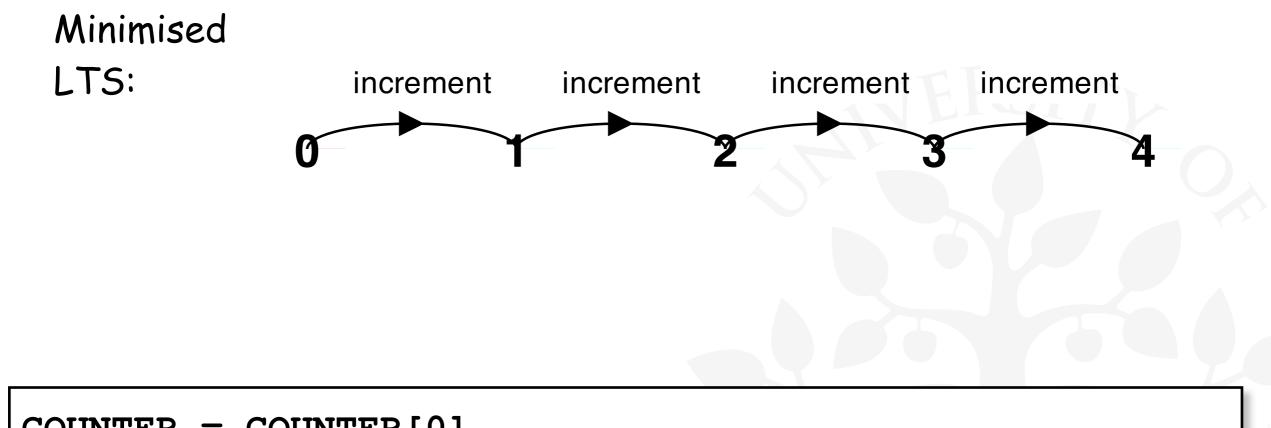
COUNTER = COUNTER[0] COUNTER[v:T] = (when (v<N) increment -> COUNTER[v+1]).
