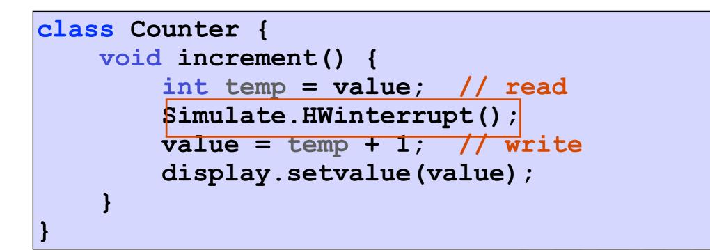
The counter simulates a hardware interrupt during an increment(), between reading and writing to the shared counter value.
