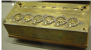
Pascals mekaniske additionsmaskine
