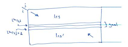
Both can be found in O(mn) time and O(n) space. Afterwards, k' can be found in a scan of the two rows in O(n) time.
