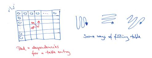
using O(1) time per table entry, hence O(mn) time in total. The value LCS(X, Y) is simply the last table entry lcs(m, n). To find this, it is enough to store  $O(\min\{m, n\})$  table entries during the execution of the algorithm, since only the last row (or column, or diagonal, depending on choice of table fill order), is needed for finding the next row. Hence, the space usage for finding the *length* of a longest common subsequence is  $O(\min\{m, n\})$ .
