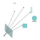
Same as finding color value for the closest triangle on the ray of the pixel (assuming this is an opaque object, and air is clear).
